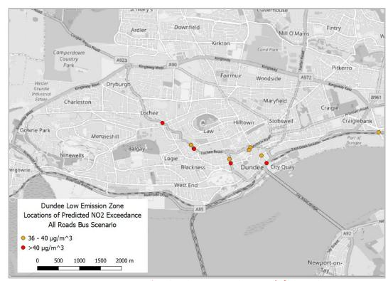
Figure 5.4 : Locations of predicted NO₂ greater than 36 μg/m³ – Bus only
