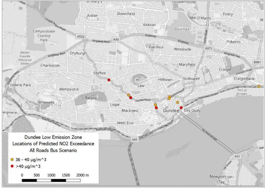
Figure 7.11 : Locations of predicted NO<sub>2</sub> greater than 36 μg/m<sup>3</sup> – NMF bus only scenario
