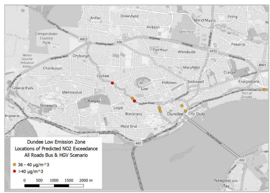
Figure 5.6 : Locations of predicted NO₂ greater than 36 μg/m³ – Bus & HGV
