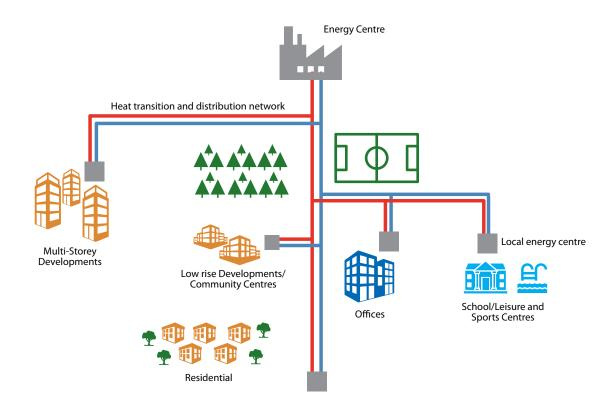
Whilst the scope of district heating projects can vary considerably, the vast majority of heat networks in the UK are relatively small-scale; in which these elements are under a high degree of common ownership or control. In many cases, generation, transmission and management is carried out by a single organisation supplying properties on a single site, typically a local authority or housing association.
