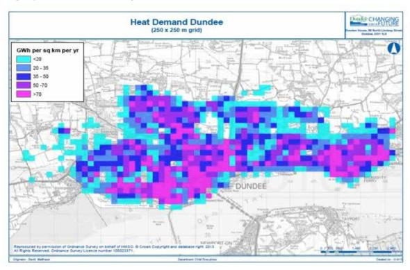
Heat mapping provides a fundamental tool in this process by providing valuable information on current heat loads within the city. It can also assist in delivering projects on the ground by modelling future heat supply and demand scenarios for investment in new developments. It will provide a means for the Council to identify links between heat sources and heat demand to optimise resources and maximise investment opportunities.
