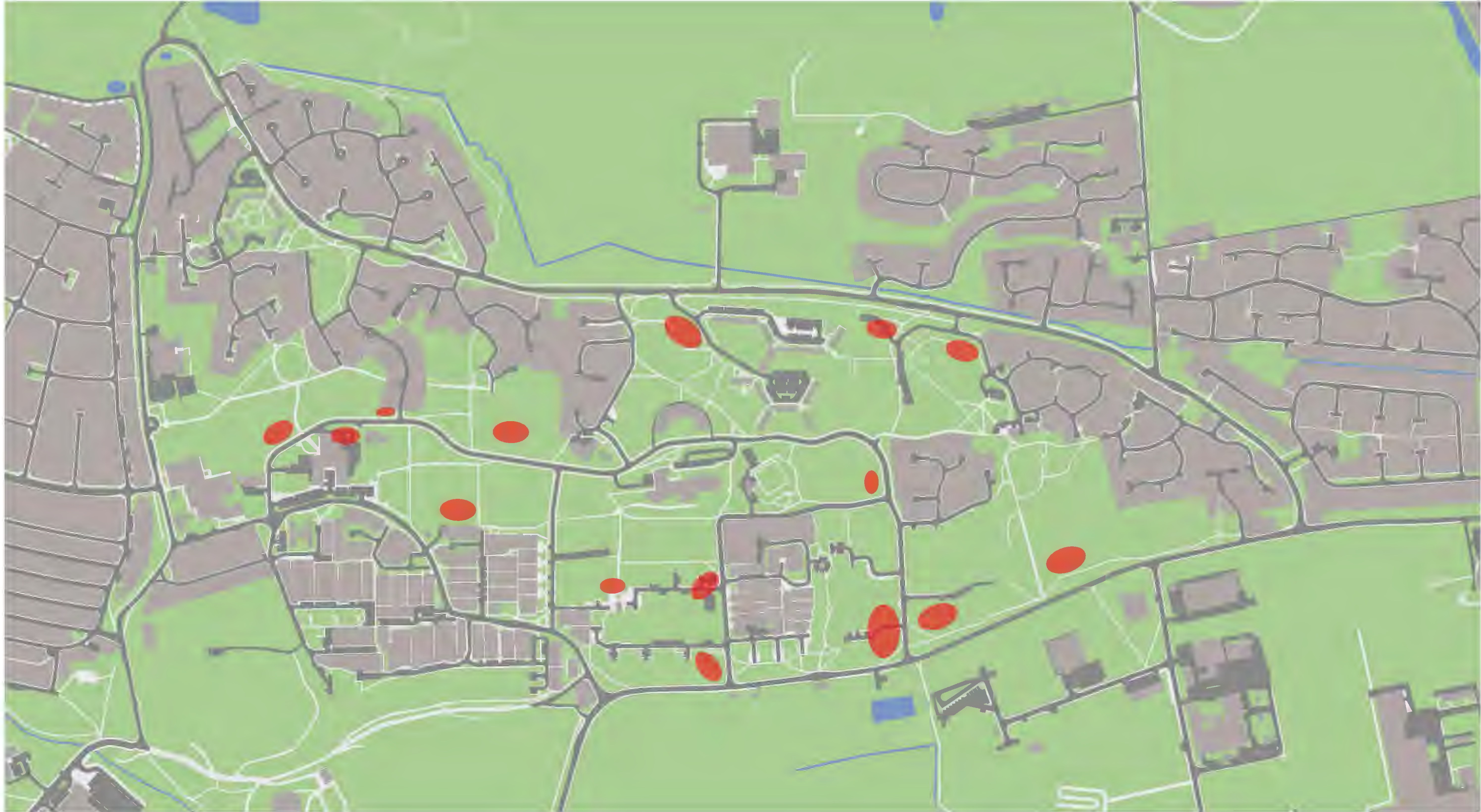
Figure 22: Map showing the potential location of SUDS basins (based on topography and other considerations) as part of the greater drainage infrastructure of Whitfield.
