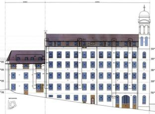
recreate a steep pitched mansard roof. The original mansard roof light pattern shall be replicated in the new roofs through the use of modern roof lights.
