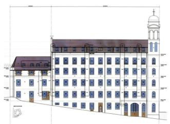
Although the roofs of the Bell, Dens Street and St Roques mill buildings will require to be replaced, the applicants propose to maintain the existing roof design through re-using the original cast iron framework to recreate a steep pitched mansard roof. The original mansard roof light pattern shall be replicated in the new roofs through the use of modern roof lights.
