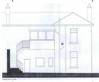
has white UPVC framed windows and grey UPVC guttering. The original cast-iron down pipes are still in place and operational.
