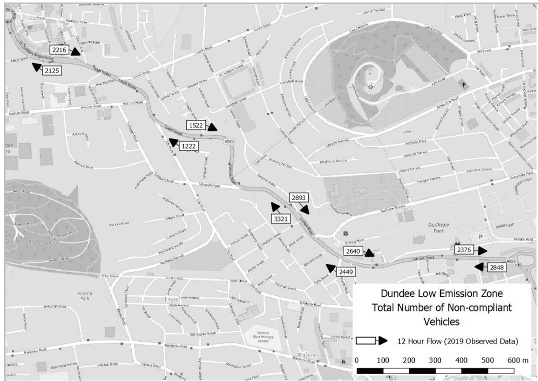
Figure 7.15 : Total non-compliant vehicles (12 hour flow) – Lochee Road
