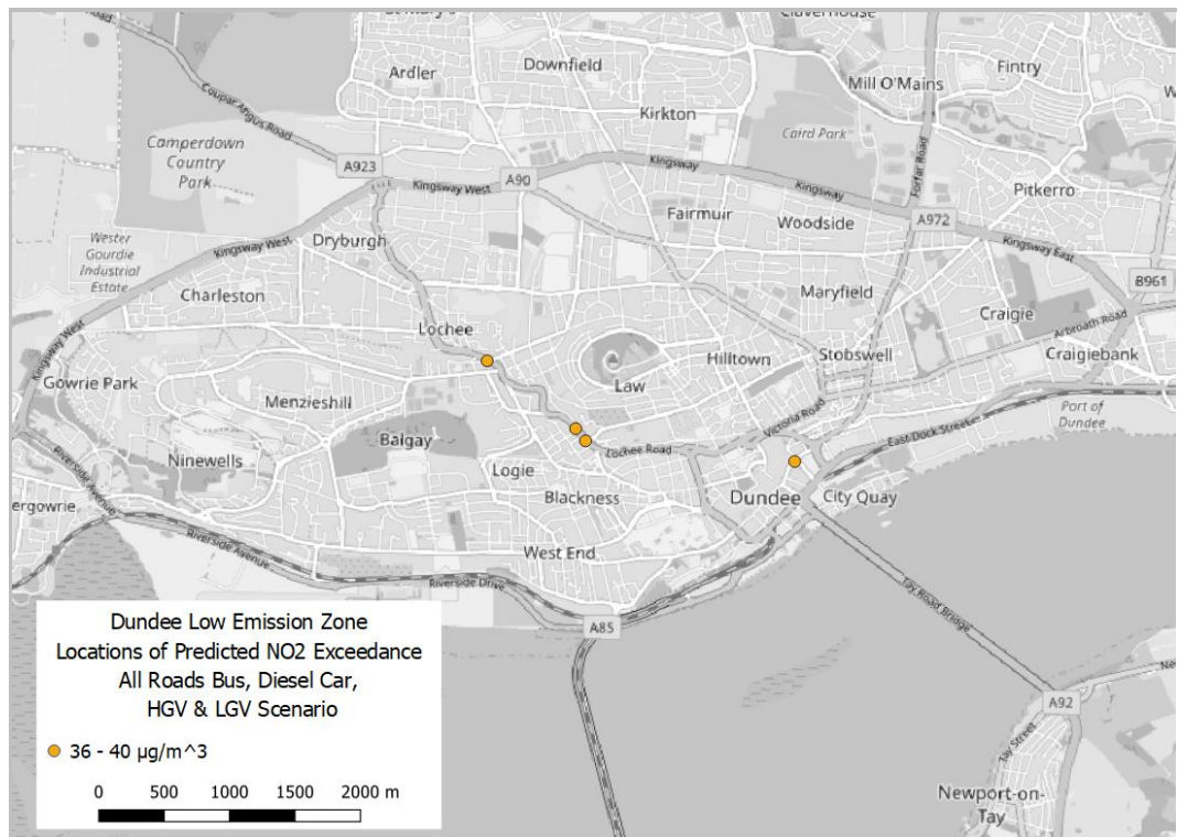
Figure 5.8 : Locations of predicted NO 2 greater than 36 µg/m 3 – Bus, diesel car, HGV & LGV
