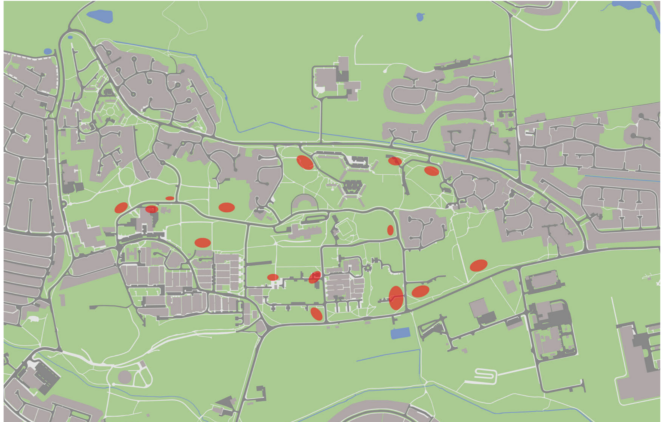
Figure 15: Map showing the potential location of SUDS (based on topography and other considerations) as part of the greater drainage infrastructure of Whitfield.
