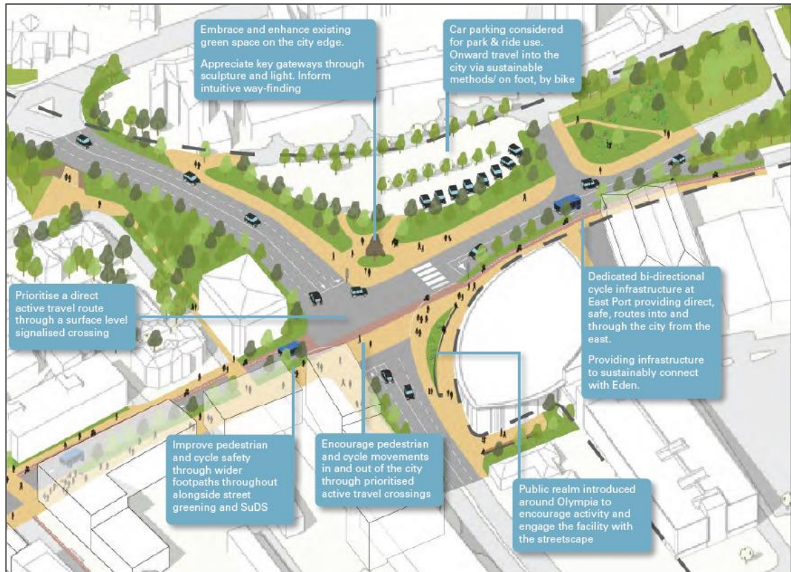
Figure 10: East Port Roundabout/Seagate proposed improvements
