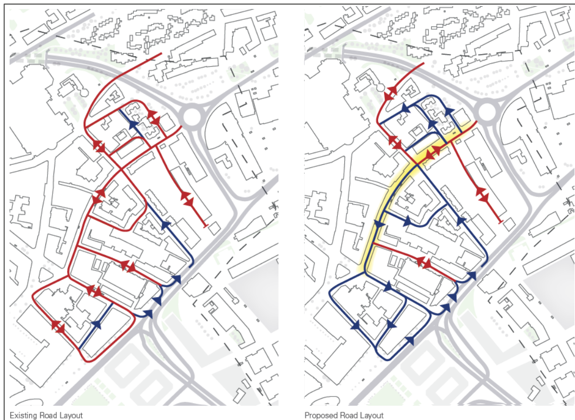
Figure 16: Seagate (Southeast quarter) proposed vehicle circulation
