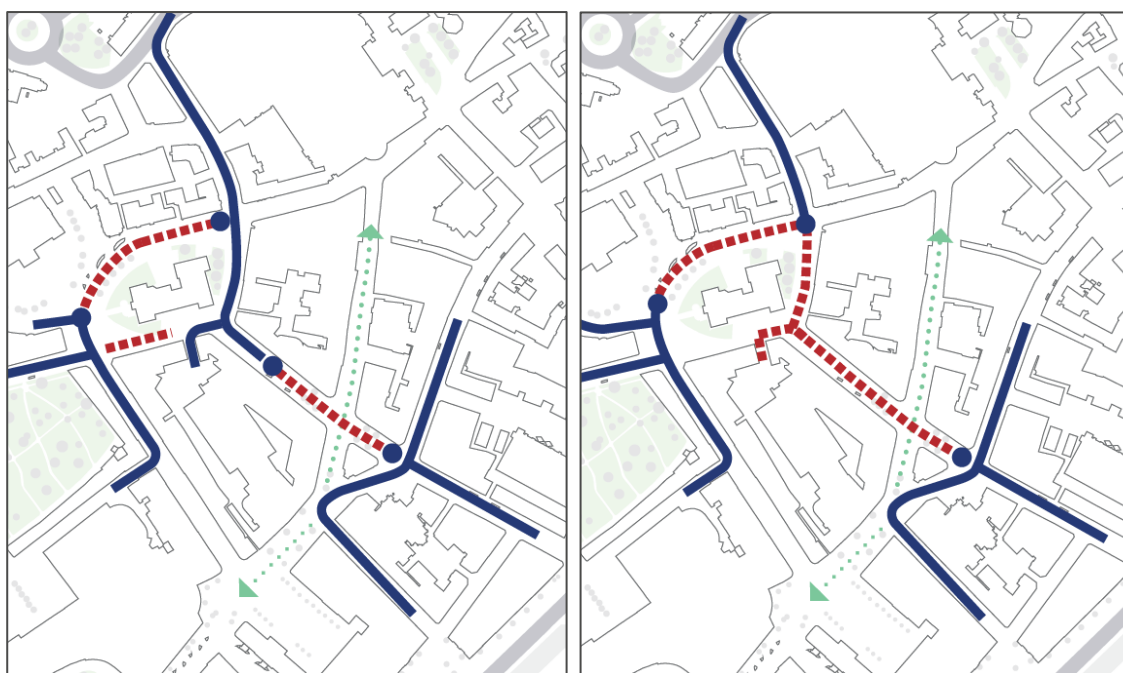
Figure 17: Existing and Proposed Road Layout at Commercial Street and Murraygate
