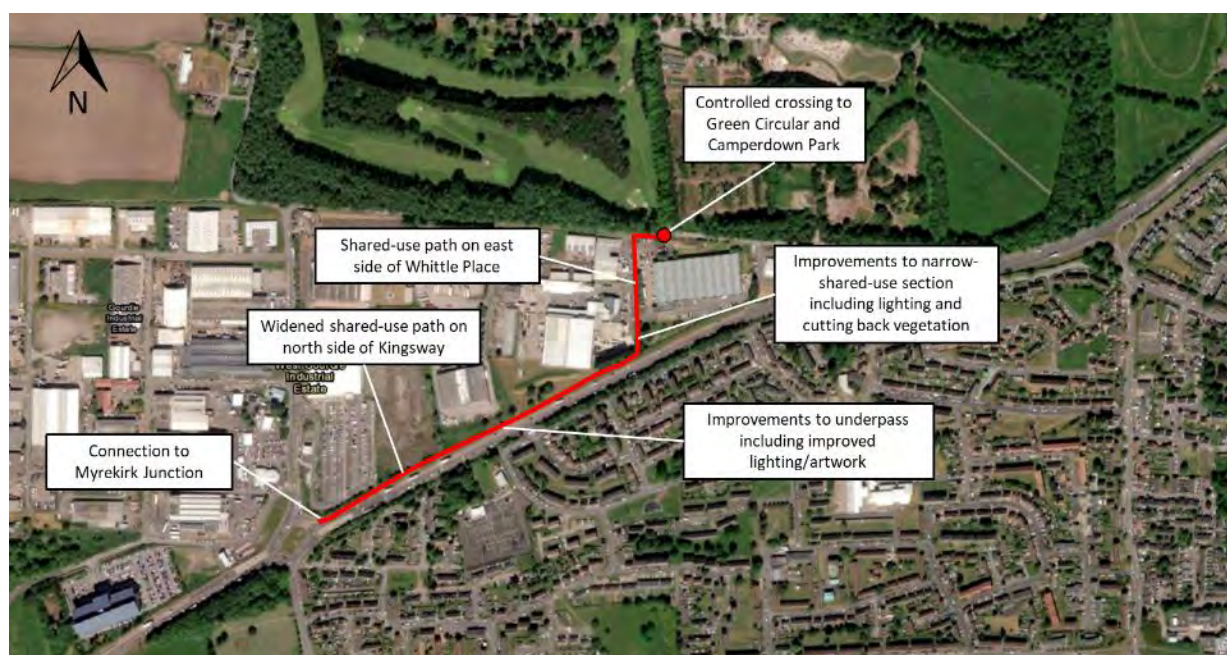
Figure 4-20 - Option E1e: Liff Road to Myrekirk Junction, Widened Shared-Use Path (Alternative to Two-Way Segregated Cycleway)
