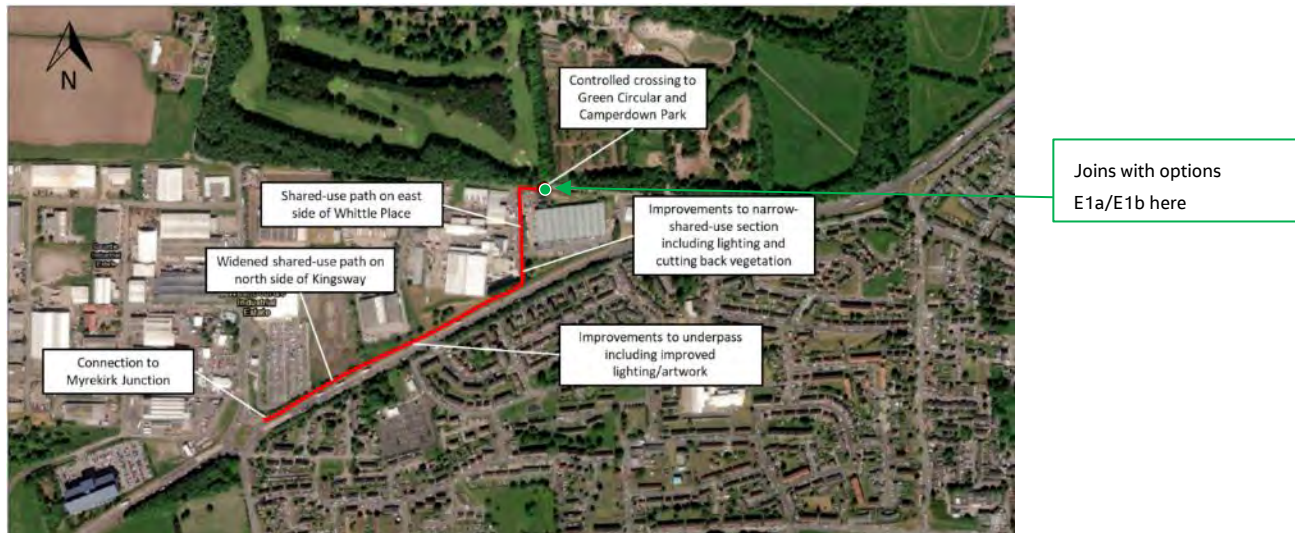
Figure 6-7 - Option E1e: Liff Road to Myrekirk Junction, Widened Shared-Use Path (Alternative to Two-Way Segregated Cycleway)
