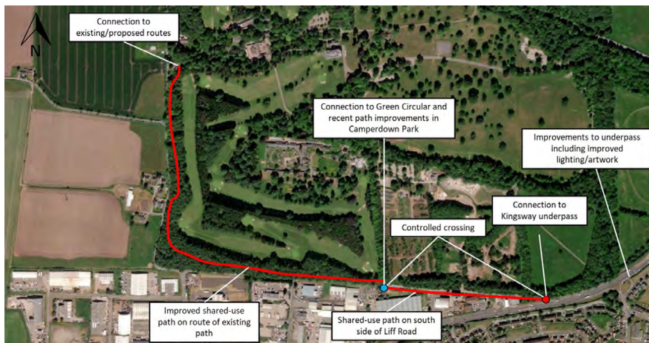
Figure 4-17 – Option E1c: Liff Road to A90 Kingsway Alternative Route, Improved Shared-Use Path Camperdown Park
