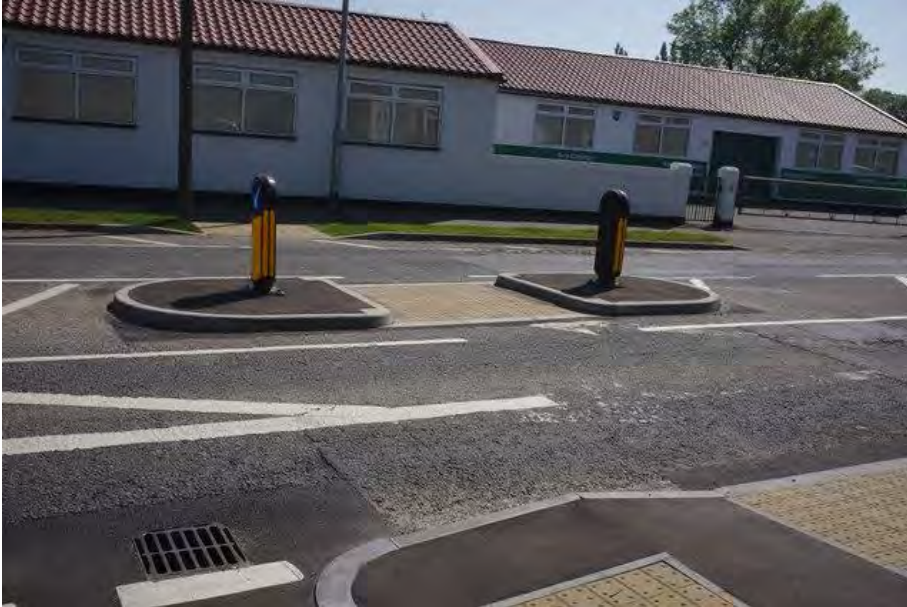
Figure 4-25 - Example of uncontrolled crossing 10
