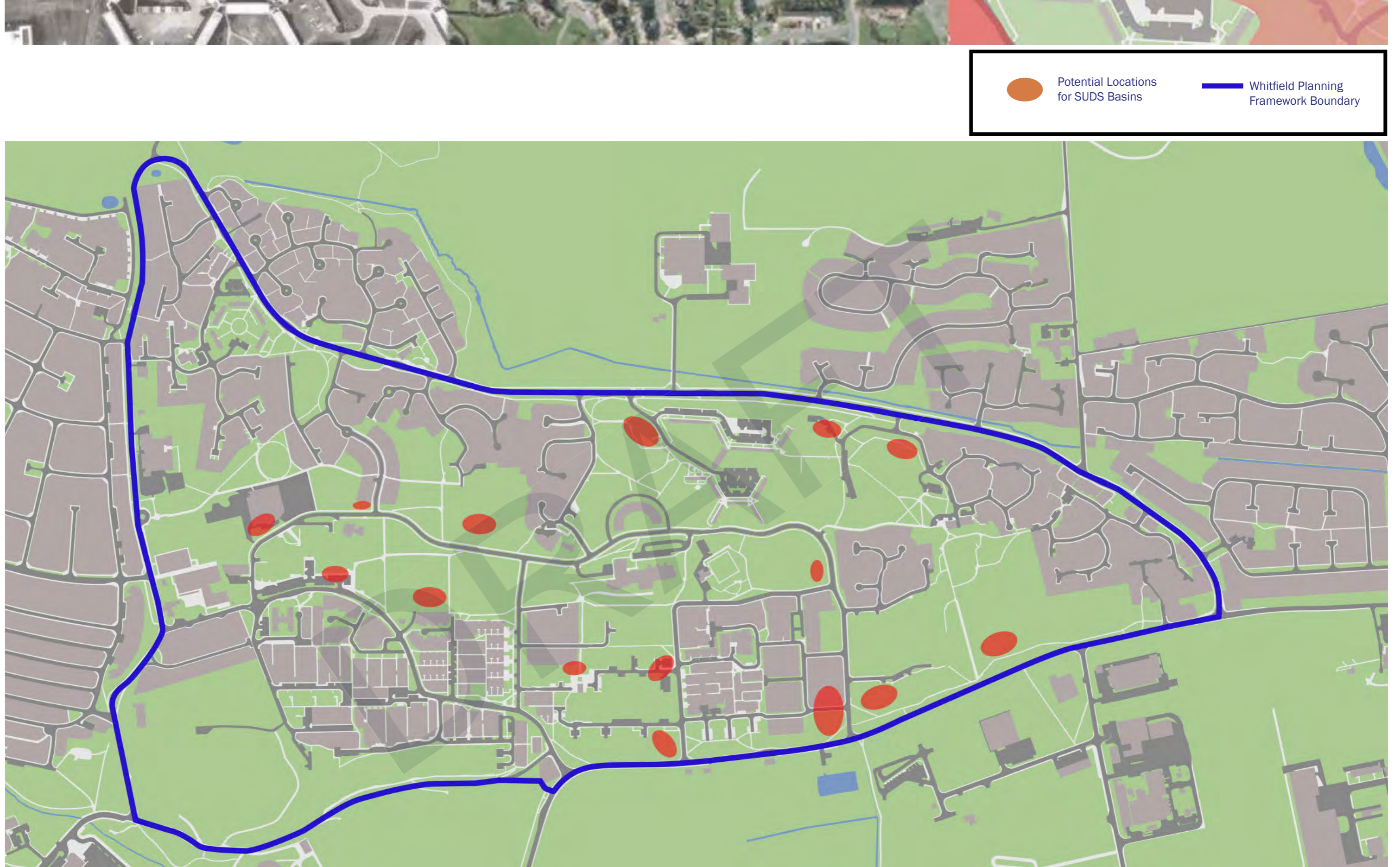
Figure 23: Map showing the potential location of SUDS basins (based on topography and other considerations) as part of the greater drainage infrastructure of Whitfield.
